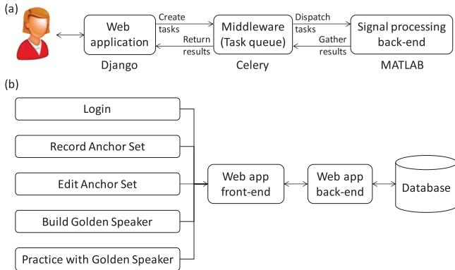
**Fig. 1.** (a) Overall software architecture. (b) Architecture of the web application.
