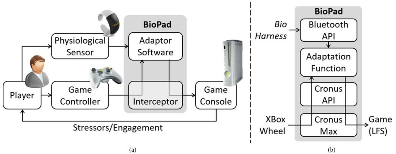
Fig. 1. (a) Hardware setup: signals from the game controller are intercepted and adapted based on the player’s physiology. (b) Control software and APIs.
