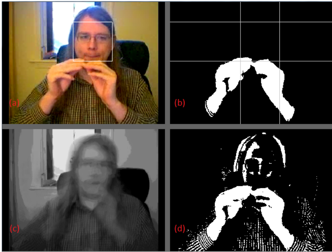
Figure 3. (a) the incoming frame of the video, (b) the final foreground image, (c) the actual background model and (d) the intermediate foreground image
