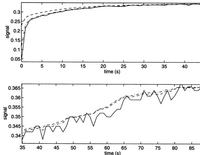
Fig. 4. Low-pass filtering of real data (solid) with an RC filter (dashed) and a decreasing cutoff RC filter (dash-dotted).
