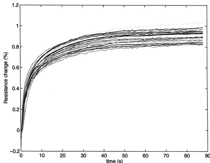
Fig. 1. Typical response of an array of 32 conducting-polymer gas sensors.
