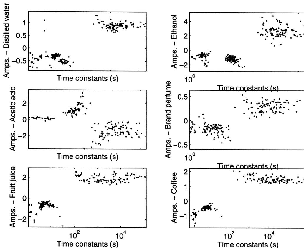
Fig. 10. Lifetime-fraction scattergrams for the Pade-Laplace method.
