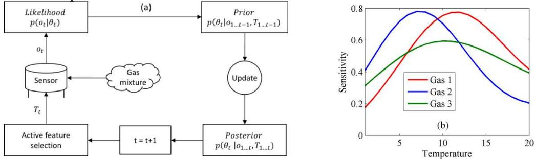
**FIGURE 1. (a)** Recursive Bayesian estimation combined with an active feature selection strategy to estimate the concentrations of a gas mixture. **(b)** Sensitivity of the MOX sensor to three hypothetical chemicals as a function of temperature.
